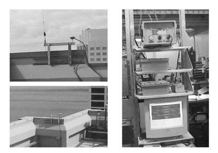
**Figure 7.** GPS and radio modem antennas at the diagonal corners of the building and the PC receiving streams of GPS and accelerometer data in real time. Shown above the PC are the accelerograph recorder and the GPS Rover units.
