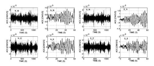
**Figure 9.** Remotely triggered and recorded accelerations at N (north) and S (south) locations. The figure shows pairs of 1200-second-long (and 60-second window from the same) record.
