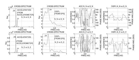
Figure 11. Cross-spectra (Sxy) and associated coherency and phase angle plots of horizontal, parallel accelerations and displacements.
