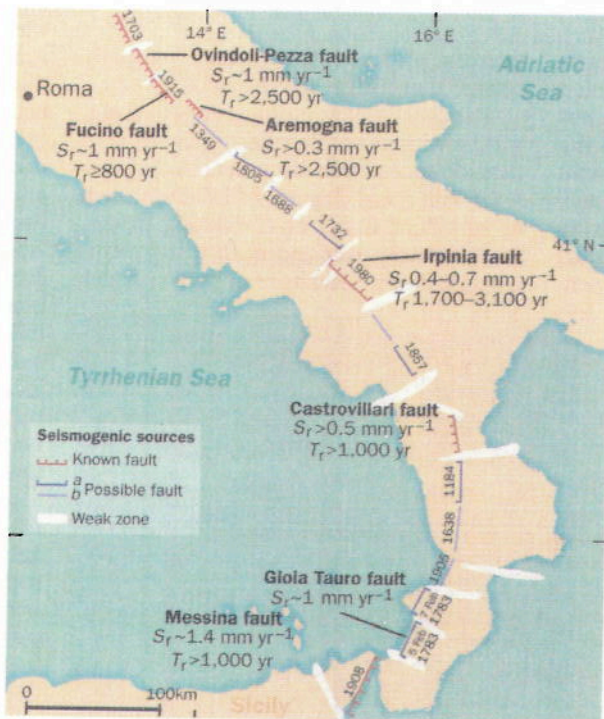
Fault segmentation, slip rate ( S_r ) and earthquake recurrence time ( T_r ) along the central and southern Apennine chain, Italy. Faults known from field observations or inferred from instrumental data are in red. Faults inferred from geological or historical data are in purple (a, high confidence level; b, low confidence). Shading marks weak zones with moderate seismogenic potential. Dates, where given, are for the last known event. (Courtesy of the Istituto Nazionale di Geofisica, Rome.)
