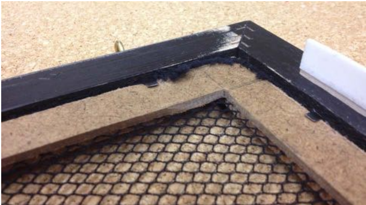
Figure 5: Frame holding the stocking (now shown in brown made from wood) emplaced in the picture frame using the metal tabs. The hook is also shown which is used to pull the frame along the track.
