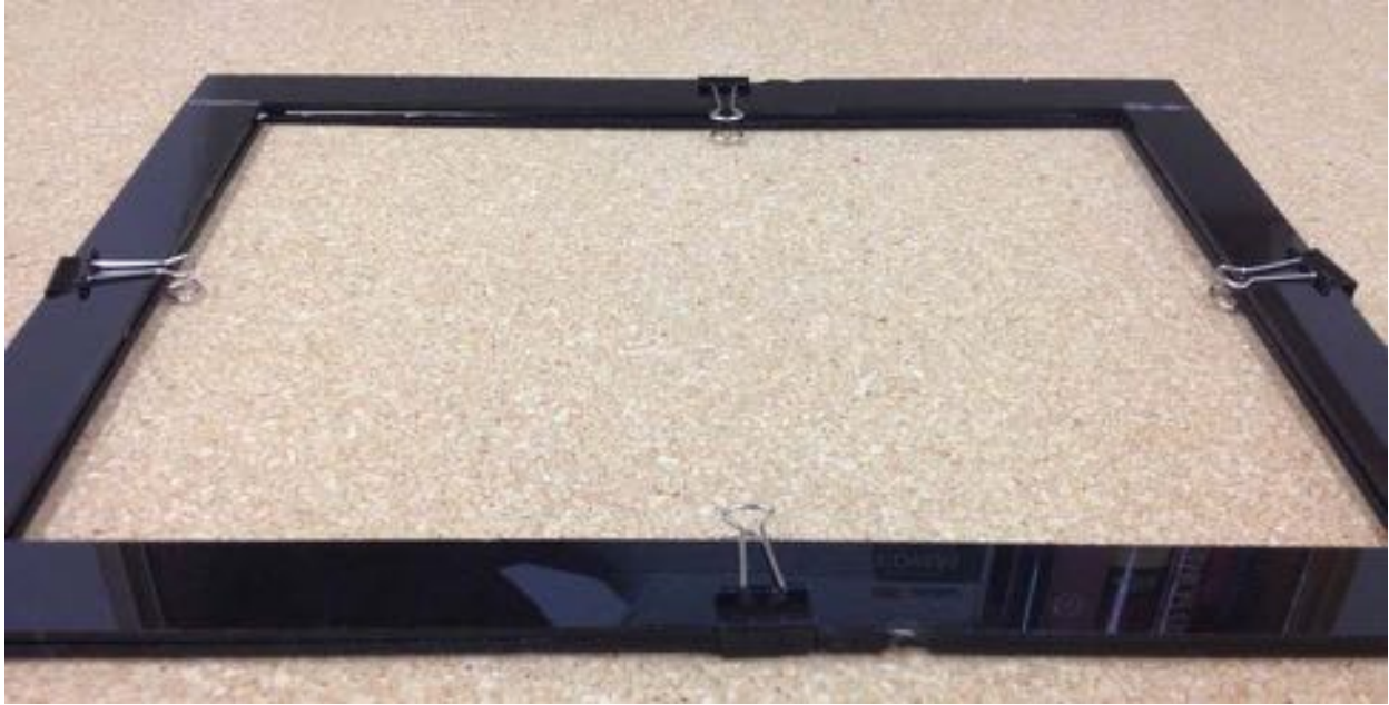
Figure 4: The two assembled acrylic frames held together by double sided tape and paper clips. The stocking has been removed from this example.
