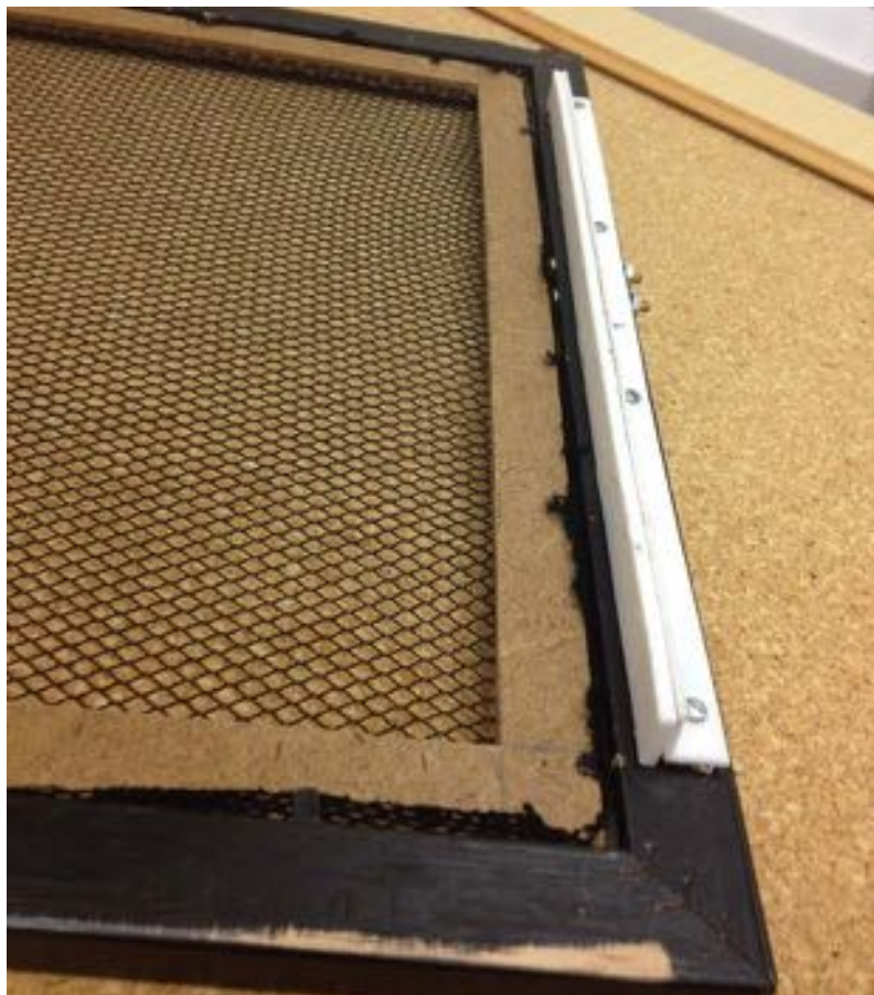
Figure 2: Teflon rails attached to the picture frame. The other side of the frame has a mirror image of this.
