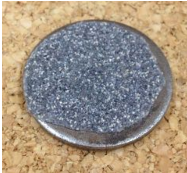
Figure 9: Single washer with non-skid attached to one side. The opposite side has duct tape ensuring the magnet will not fall out.
