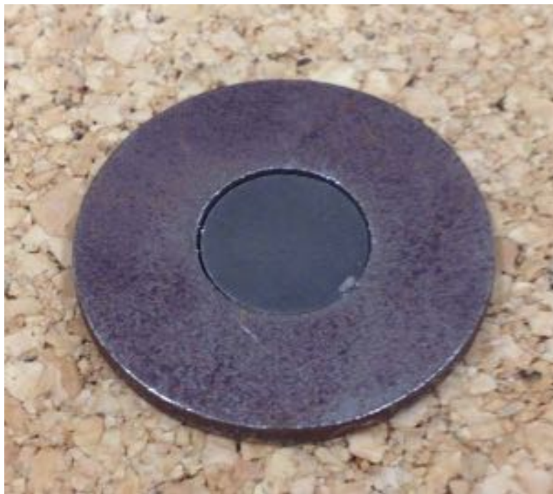
Figure 7: Neodymium magnet placed in the washer. The opposite side has been hammered in to prevent the magnet from falling out.
